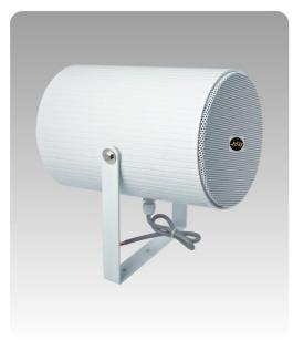
The built-in two 6" full range speaker drivers are designed of wide frequency response 110-15kHz, the multiple power taps 5W, 10W & 20W are helpful for different applications varies from room size and ambient noise surroundings.
